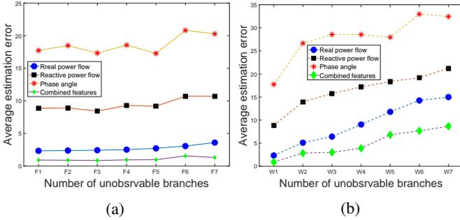
Fig. 4: Average estimation error using different features a) randomly scattered attack, b) localized attack.
