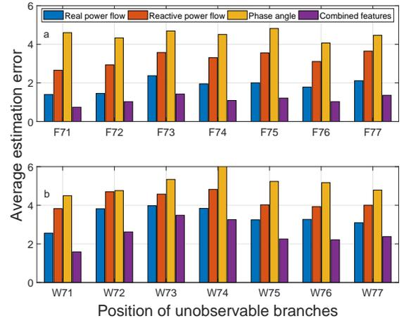
Fig. 6: Average estimation error for a) randomly scattered attack (F7), b) localized attack (W7) using different features.
