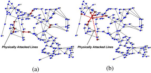
Fig. 2: Example of a) scattered attack scenario, and b) a localized attack scenario. The red marked branches have experienced cyber attack and became unobservable and the red dashed lines indicate branches, which are physically attacked.
