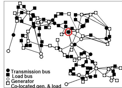
Fig. 1: The IEEE 118 bus system topology with its control center marked with a circle.
