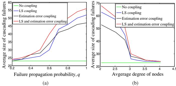
Fig. 3: Average size of cascading failures (number of tripped lines) a) as a function of  $q$  and different levels of coupling between the power system and the communication network, and b) as a function of average degree of nodes in the communication network for  $q = 0.5$ .
