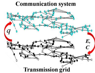
Fig. 2: Schematic depiction of the coupling effect between the power grid and its communication system.
