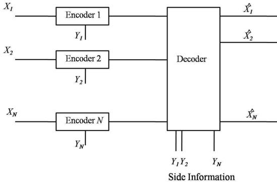
Fig. 4. The proposed distributed source coding model with side information to characterize the control overhead.
