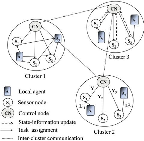
Fig. 1. A sensor system and its clusters.
