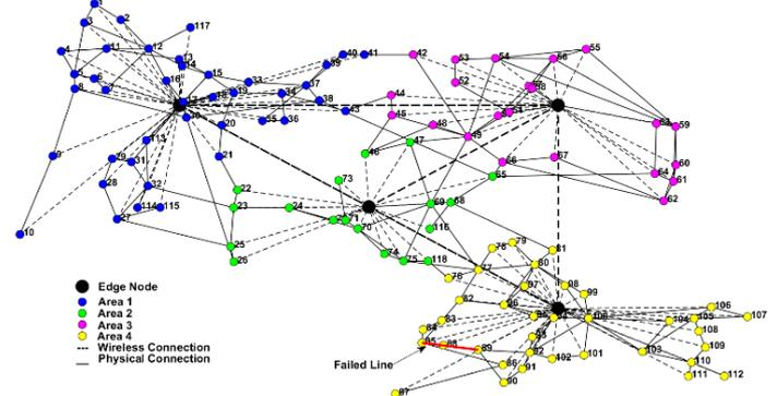
Fig 2: Simulation schematic of event detection based on Edge-enabled EGT over IEEE 118 bus system.
