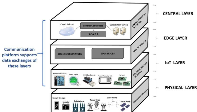
Fig. 1. Layers of the edge-enabled IoT for smart grids.
