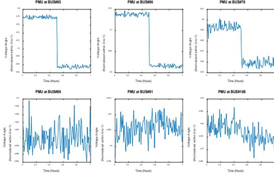
Fig. 3: Examples of the effect of a line trip on some of the PMU time series connected to the edge node  $E_4$ .
