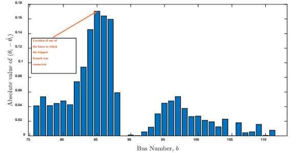
Fig. 5:  $\theta_b(t_a) - \hat{\theta}_b(t_a|t_a-1)$  for all the PMUs connected to edge node  $E_4$ .
