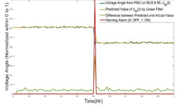
Fig. 4: The alarm for anomaly. Only one PMU data has been shown for better visualization.
